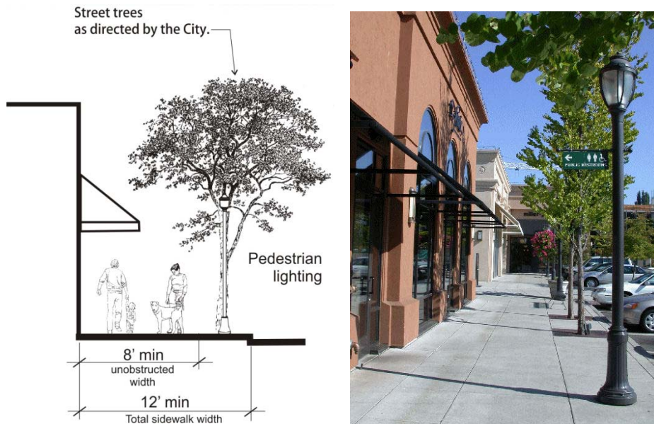
Figure 18.120.030.B.2.c Left: Illustration of requirements for a building front facing a parking area. Right: Example of a successful pedestrian sidewalk between parking lot and storefront.
