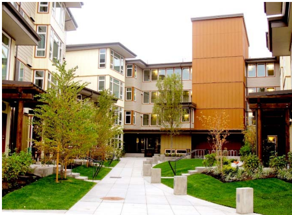
Figure 18.120.020.C.2.a. A good example of pedestrian connections between units. The pathway leads to the street. Note the positive security measures including bollard lighting, open landscaping with no hiding spaces, passive surveillance from windows and sense of enclosure that implies ownership of the space.
