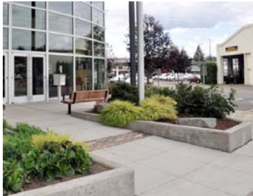
Figure 18.120.030.D.2.g. Plant beds in front of City Hall. Note the raised beds that enable easy maintenance and the bands of ornamental pavement.
