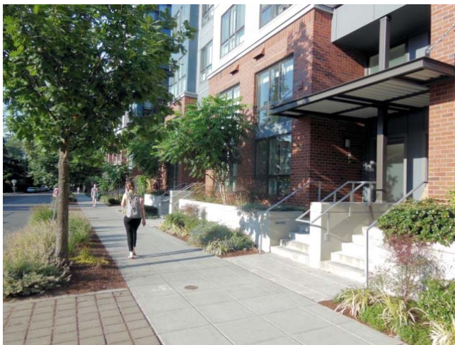
Figure 18.120.020.B.3.e Desirable ground related residential example with raised unit, landscaping and small porches to enhance privacy while providing a welcoming streetscape. Units front on the street. Garages are off the alley.
