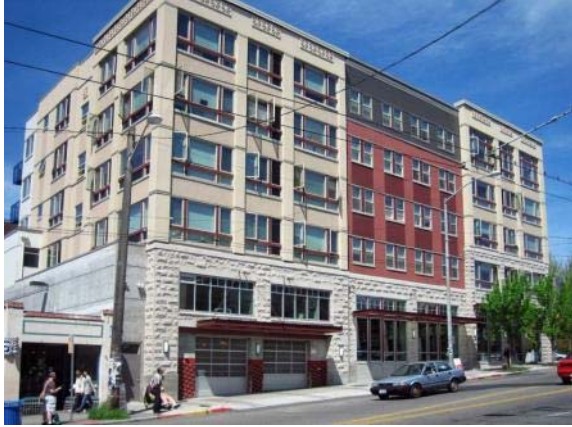
Figure 18.120.040.D.2.d. Example of a architecturally dividing a façade into sections that give the impression of a composition of smaller buildings.
