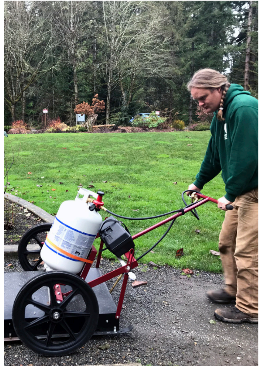
Park Maintenance Staff Member using a flame weeding tool.
