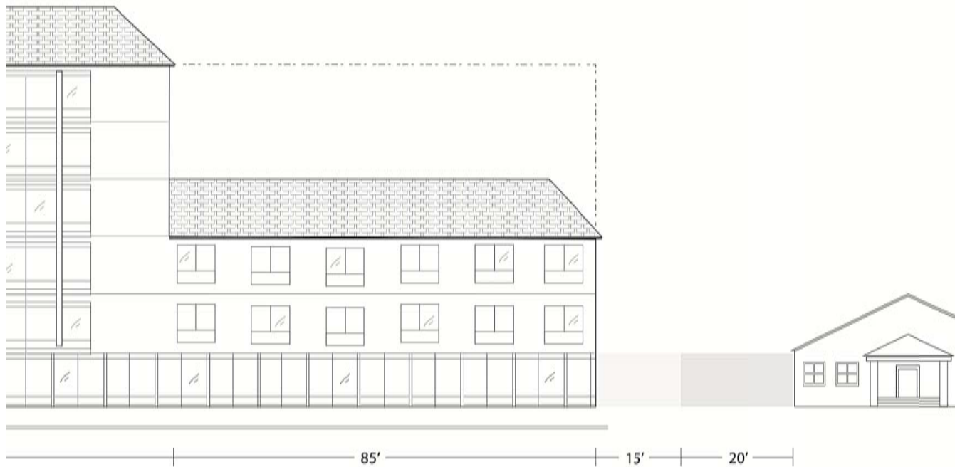
Example of proposed 'Stepback' adjacent to low density (14 or less housing units per acre) zone
