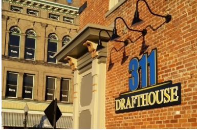
Sign with External Lighting
