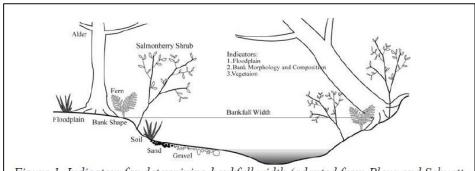
Figure 1. Indicators for determining bankfull width (adapted from Pleus and Schuett-Hames, 1998).
