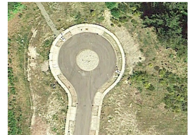
Cul-de-sac built to current City of Olympia Standards.
