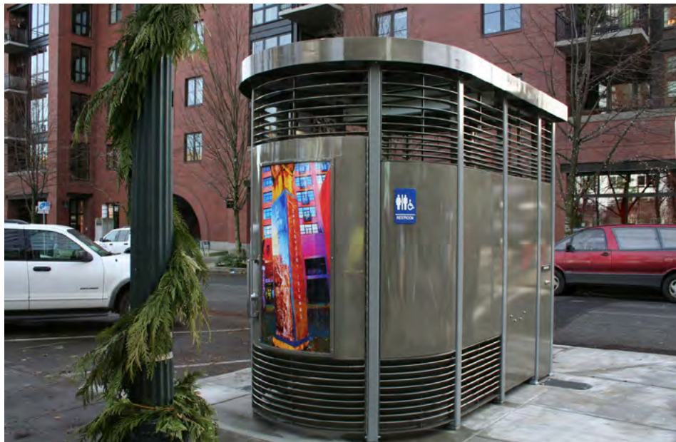
Similar challenges in Portland Oregon led the City to develop and build the Portland Loo, that features enough privacy for human dignity, while maximizing visibility to deter negative behavior.
