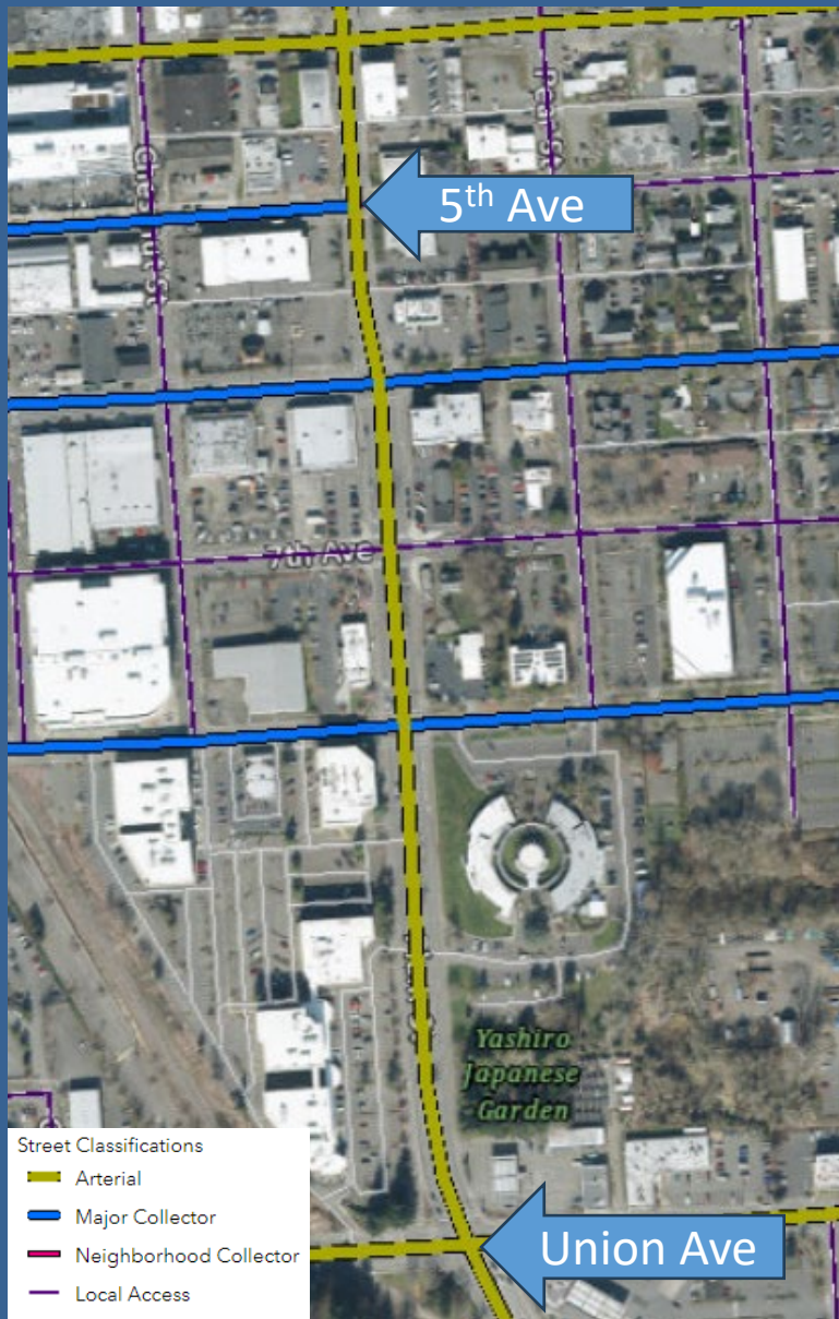
Street Classifications as designated under Engineering Design and Development Standards Chapter 4 - Transportation
