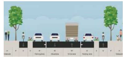
Figure 4-7. Typical street standard option for new essential streets. Some of the first new developments could make use of public funding to meet street requirements.
