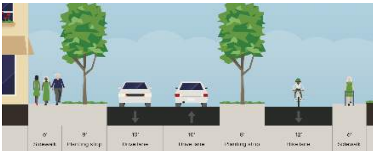
Figure 4-6. 4 th Avenue shared use path, landscape, and low impact development (green stormwater infrastructure) conceptual vision.
