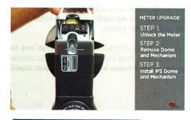
3. Install IPS top cover (dome) and insert IPS coin/credit card/wirelessenabled mechanism.
