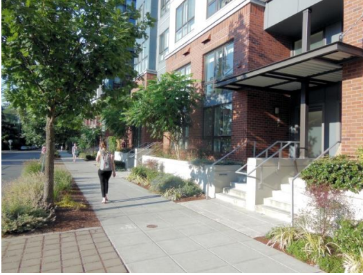
Figure 18.120.240.A.1: Desirable ground related residential example with raised unit, landscaping, and small porches to enhance privacy while providing a welcoming streetscape. Units front on the street. Garages are off the alley.
