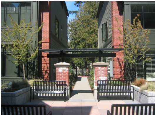
Figure 18.120.280.B.5: Note the use of both territorial definition in the foreground seating area and access control in the gate towards the rear of this picture. The gate, even if unlocked, indicates that the courtyard in the background is private while the benches indicate that people are welcome to use the courtyard in the foreground.
