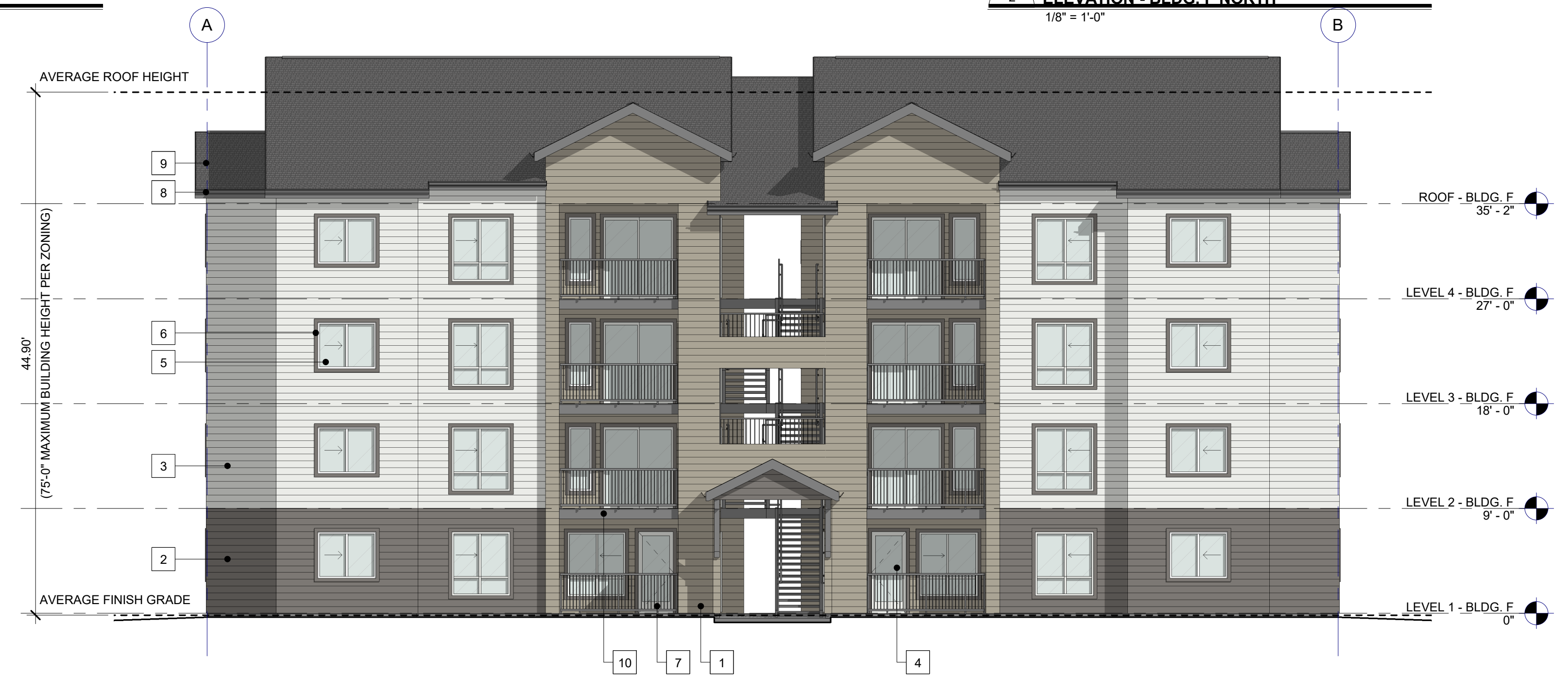
ELEVATION - BLDG. F WEST 1/8" = 1'-0"
