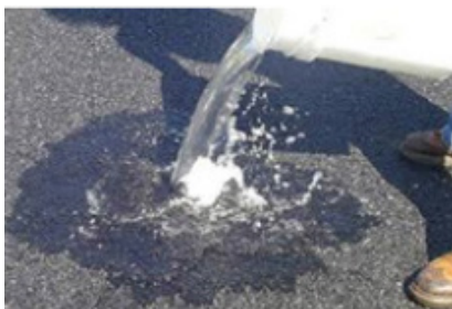
Increased erosion and sedimentation prevention is needed for permeable paving to prevent plugging and reduction of infiltration (Element 14).
