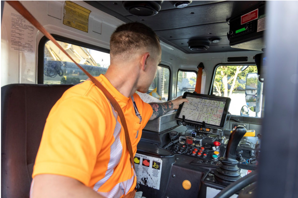
Figure 23 Collection Driver Using GIS Routing with Tablet
