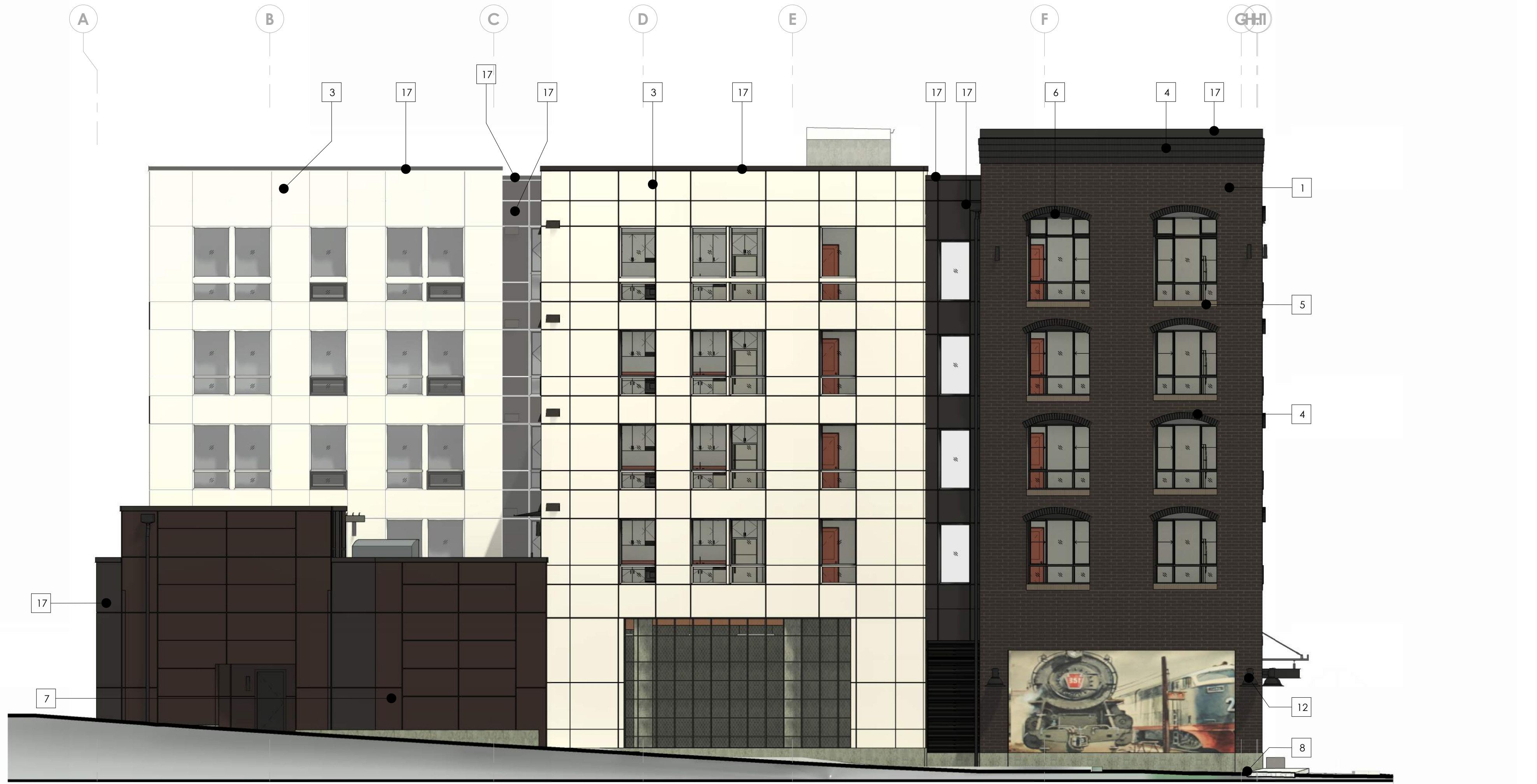
1 SOUTH ELEVATION DRB 1/8" = 1'-0"
