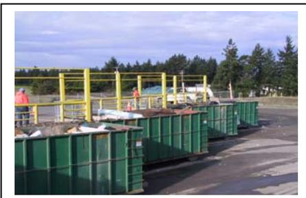
Most non-commercial haulers with MSW and general debris are directed to the self-haul tipping area, consisting of a z-wall equipped with 10 drop boxes which can be used by up to 10 to 15
