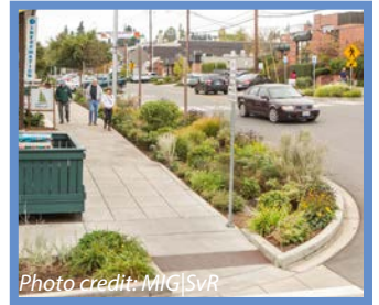
Curb bulbs slow traffic at intersections, shorten the crossing for pedestrians, and provide space for landscaping or other amenities.
