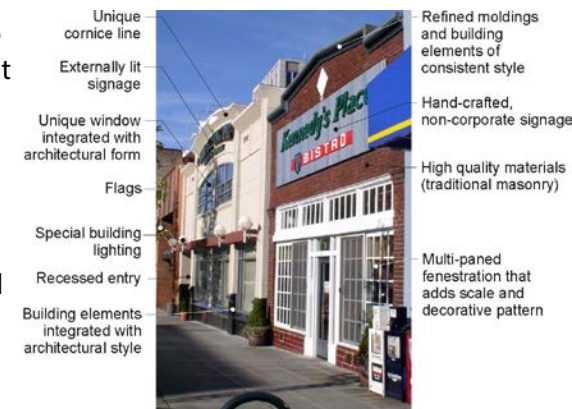
Building design guidelines that emphasize pedestrian interest, small scale street facades, and diversity
