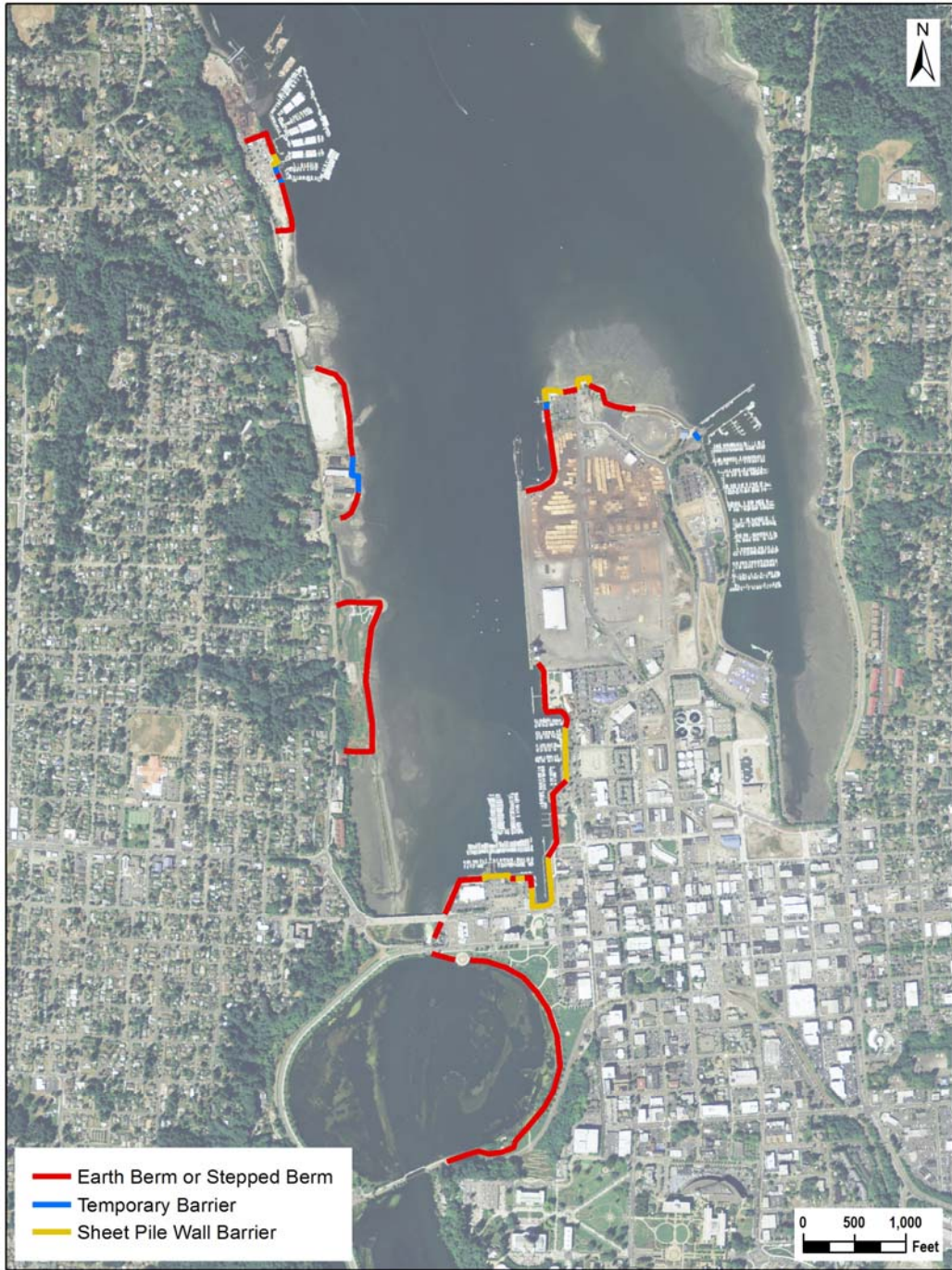
Figure 44. Barrier location for flood protection at 0.25 ft and 50 inches sea level rise
