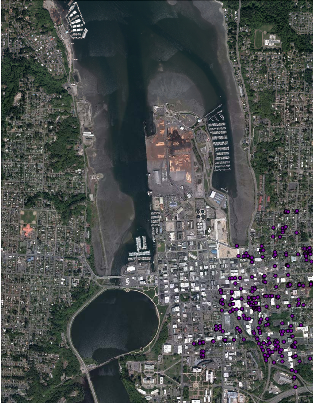
Figure 17. Hydraulic model nodes at catch basin locations of 72-inch pipe system
