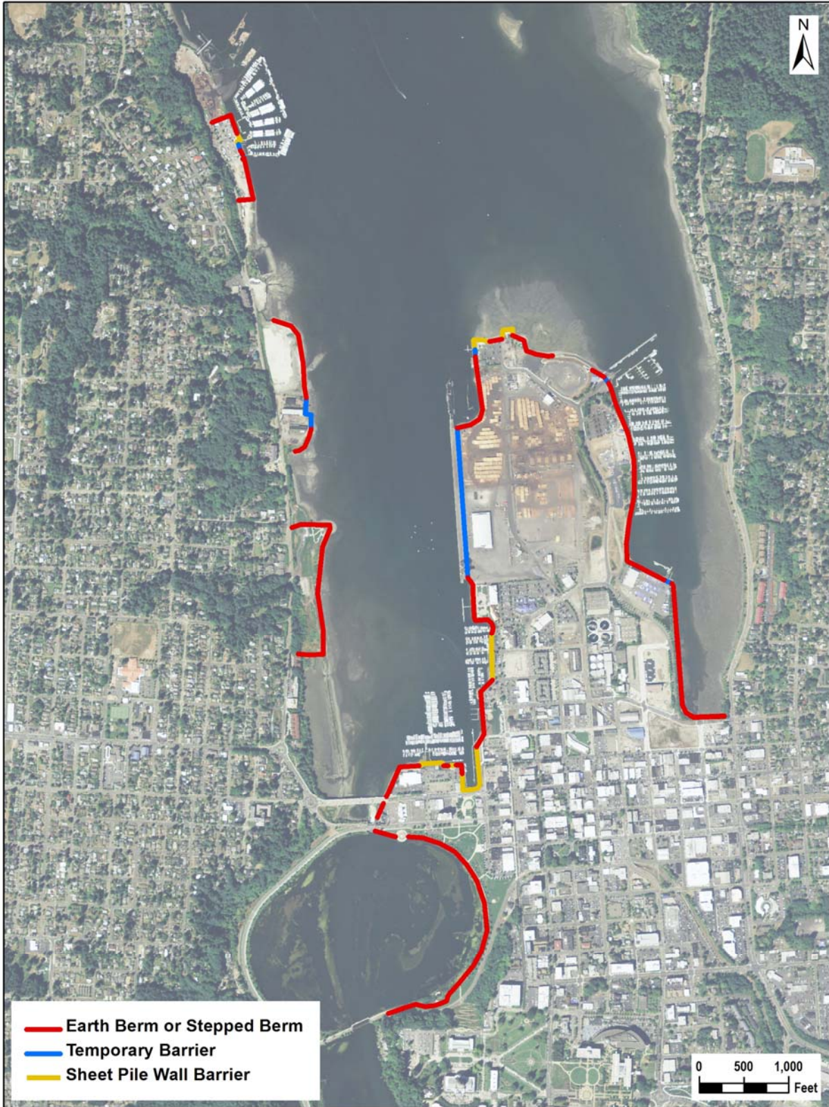
Figure ES-2. Flood barrier locations to protect Olympia at 0.5 ft sea level rise
