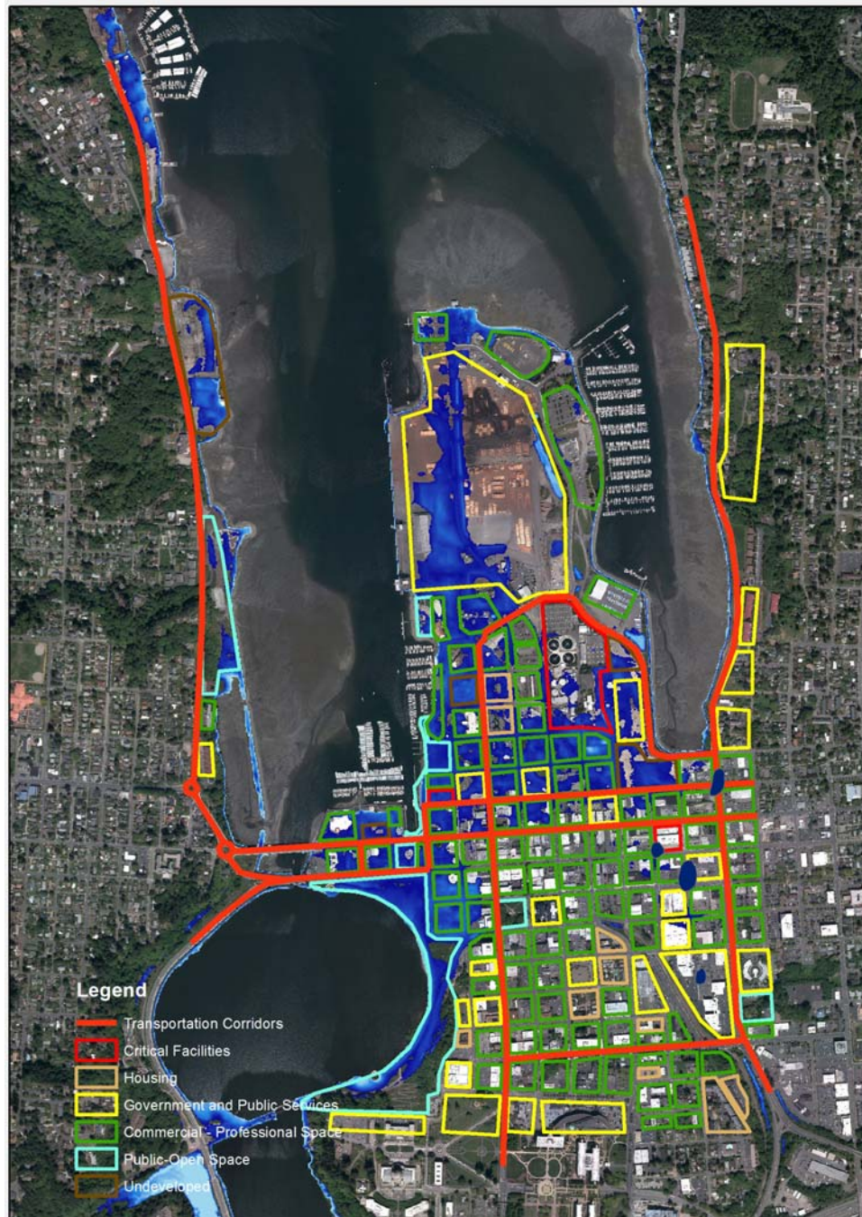
Figure 29. Land use categories and essential transportation corridors with inundation limits of 100-year total water level, existing sea level
