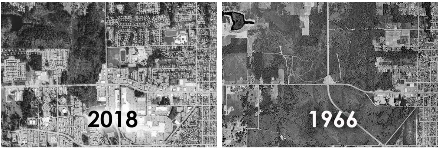
Pull the slider back and forth across the image to see impervious coverage on Olympia's west side in 2018 and 1966.
