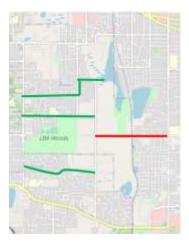
Each of these three Major Collector connections can carry about 10,000 vehicles per day in the current configuration. The current traffic on Herman Road is less than one-third of this amount.
