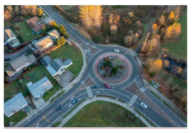
The roundabouts on Boulevard Road have kept traffic moving as the area has grown, allowing Boulevard to remain a two-lane street. The concept of concurrency means that as our community grows, we add "capacity" to the street.
