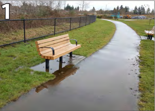
Install 36" x 48" asphalt pad next to park bench.
