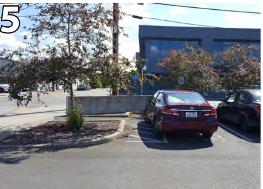
Inadequate ADA parking. Provide (3) ADA accessible parking spaces. (1) must be van accessible and have proper signage.
