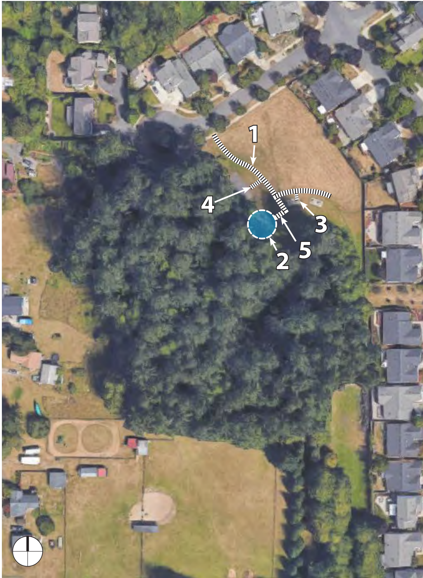
1 Existing pathway is worn and narrows to 24" for large portions of its length. Replace with ADA compliant pathway.
