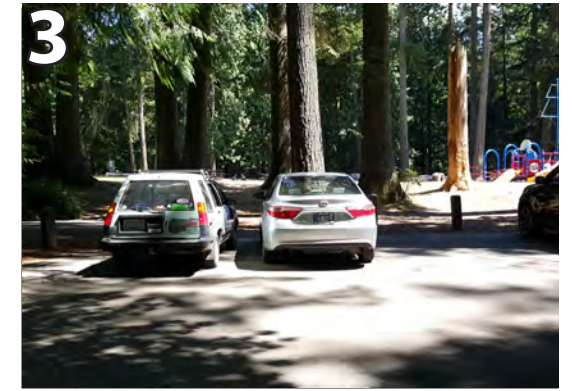
No ADA parking space for shelter #4. Re-strip to provide for (1) accessible space. Install signage
