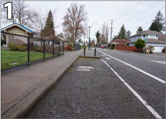
No ADA accessible parking. Install (1) van accessible ADA on-street parking space.
