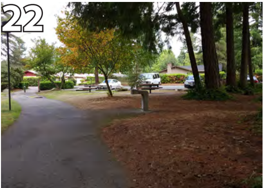
22 Area around drinking fountain too steep. Regrade with a slope no greater than 1:48.
