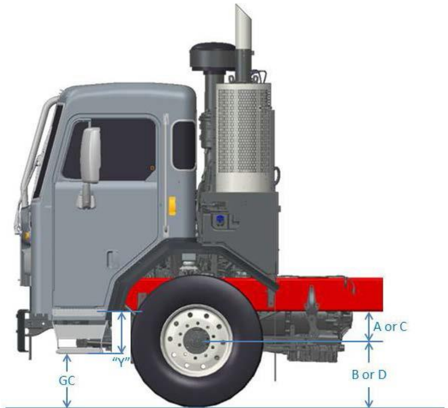
FIGURE 3-28. Ground Clearance Calculations
