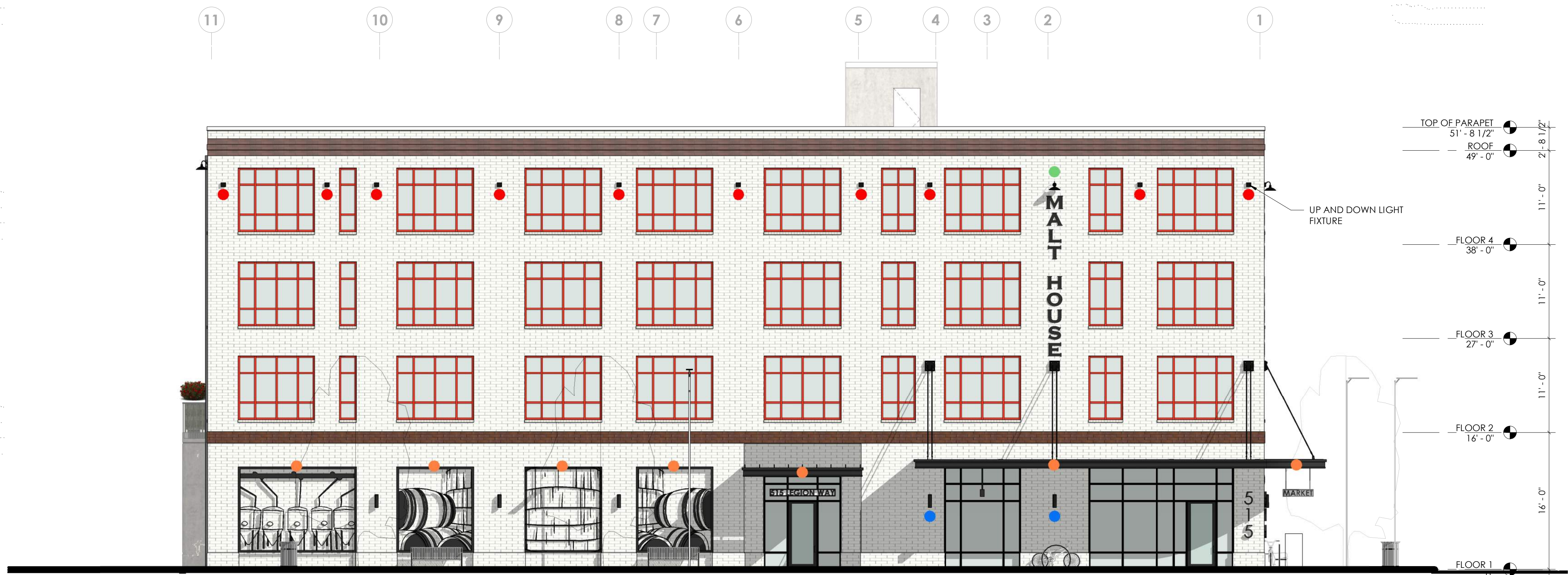
1 NORTH ELEVATION - LIGHTING 1/8" = 1'-0"
