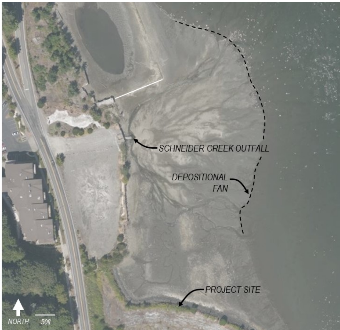
Figure 2-11: Schneider Creek outfall and its depositional fan, north of the Project Site.
