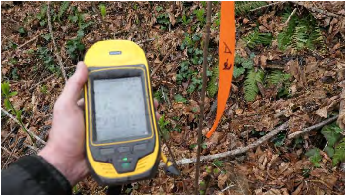
Photo 17. Record flag locations with Trimble at sub-foot accuracy
