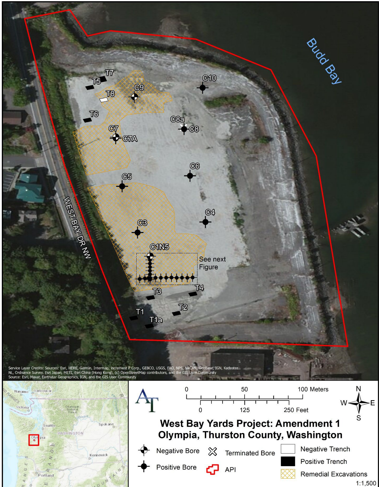
Figure 21. Location of the direct-push bores and trenches excavated across the API.
